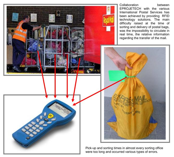
Postal services looked to resolve the problem by turning to RFID technology. Furthermore a system has also been created to verify quality of the service by inserting an UNDERCOVER BAG with another RFID chip inside the bag. The reader device can read numerous tags at the same time, in this way tracing their course. It is also possible, in the same way, to verify the transportation of the various sacks is carried out within the estimated delivery time.
