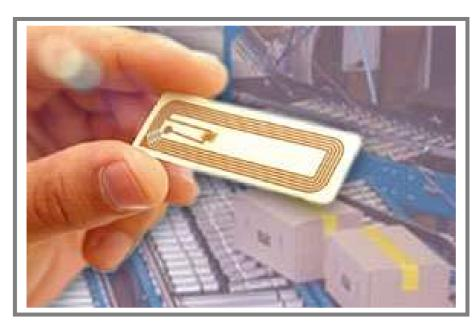
Tag Transponder & Smart Labels HF (13,56 MHz) ISO 15693 e ISO 14443 UHF (868 MHz) ISO 18000
